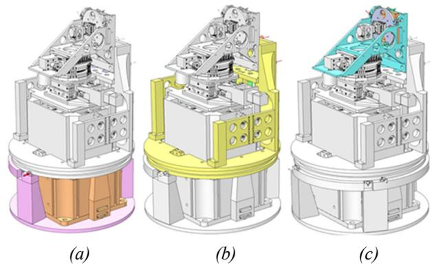
Figure 9: 3D model of the capacitive sensor metrology for scanning rotation stages (a) sample pitch stage metrology (b) linear sample scanning stages (c) sample yaw stage metrology.
