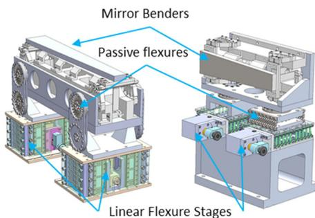
Figure 5: 3D model of horizontal and vertical KB alignment apparatuses.
