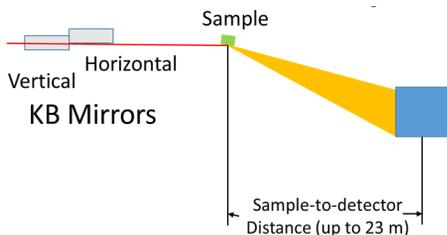
Figure 1: Instrument schematic: Not to scale.
