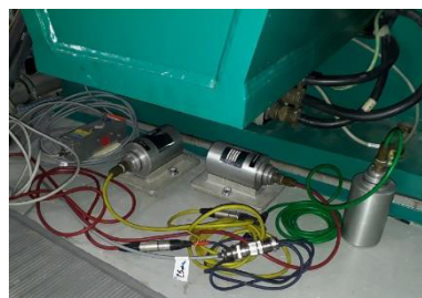
Figure 12: Velocimeters implementation on slab.
