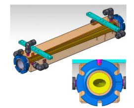
Figure 4: High power diaphragm. Insert bottom: cornerless entrance and exit window.
