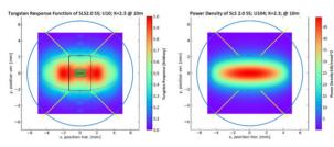
Figure 3: Example of the plots used to adjust the positions of the tungsten blades in the W-XBPMs. Left: tungsten response function plot. Right: power density plot.
