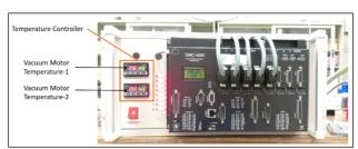
Figure 5: Temperature Controller & Motor Controller.
