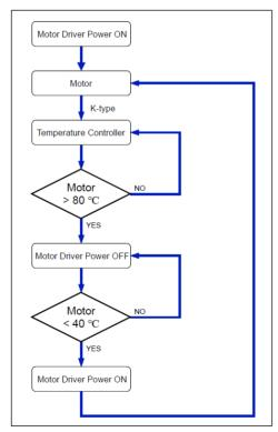
Figure 4: The temperature protection flow chart of the vacuum motor.
