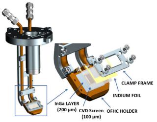
Figure 6: FSWB Cooling Flange and detail of the CVD diamond screen clamping design.
