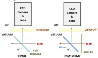
Figure 1: Geometrical configurations of the FSMs.
