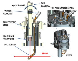
Figure 5: Imaging system and scintillator screen arrangement for monochromatic FSWB.
