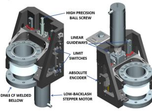
Figure 3: Motion stage assembly. FSWB and FSM2 arrangement (left), FSM1 arrangement (right).
