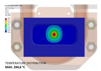
Figure 7: Temperature distribution on diamond screen.
