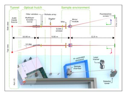
Figure 1: MINERVA layout presenting the main components of the beamline. Side view in a), top view in b) and 3D view in c).
