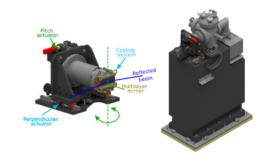
Figure 2: Monochromator mechanics description.
