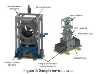
The vacuum chamber is fully decoupled of the sample positioning stages by means welded bellows with robust columns holding the in-vacuum base plate. A metallic frame around the chamber includes two autocollimators that measure the 3 orientation angles MM respect of the incident beam which signal is re-used to act on the main hexapod for orientation correction.
