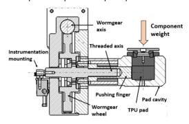
Figure 8: Cross-section of the prototype TPU pad design.
