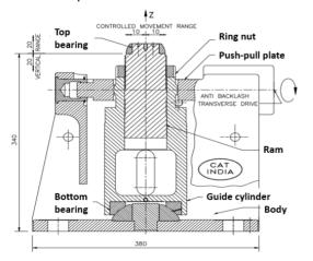
Figure 1: Transverse cross section of the LHC jack [2].
