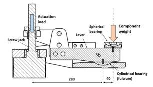
Figure 4: Cross section of the lifting lever solution.
