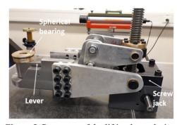
Figure 5: Prototype of the lifting lever design.
