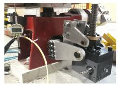
Figure 6: Prototype lever inserted in the magnet jack.
