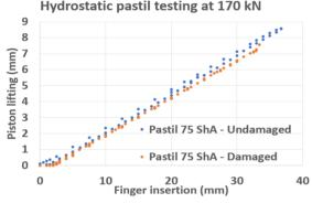
Figure 7: Testing of the 75 ShA TPU pad at deep finger insertion and high loads.
