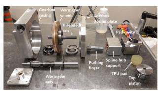
Figure 9: TPU pad prototype upon assembly.
