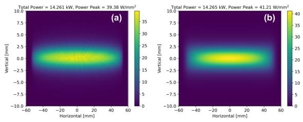
Figure 2: Power density distribution of ESRF-W150: (a) Using ray-tracing and (b) New OASYS widget Wiggler Radiation.
