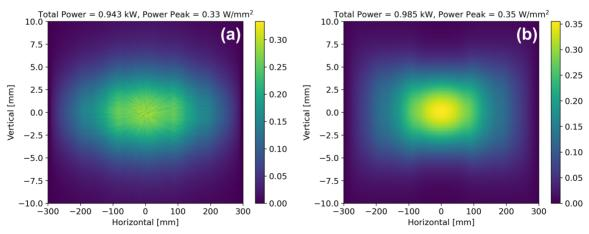
Figure 3: Power density distribution of BEATS project source: (a) Using ray-tracing and (b) New OASYS widget Wiggler Radiation.
