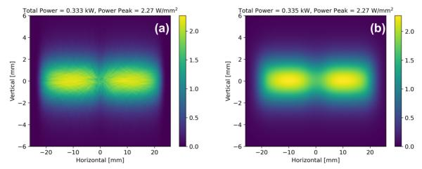
Figure 1: Power density distribution of ESRF-3PW: (a) Using ray-tracing and (b) New OASYS widget Wiggler Radiation.
