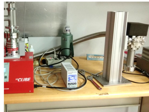
Figure 5: Photograph of the prototype sample cryogenic cooling chamber test setup.
