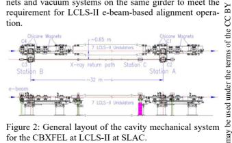
Figure 2: General layout of the cavity mechanical system for the CBXFEL at LCLS-II at SLAC.
