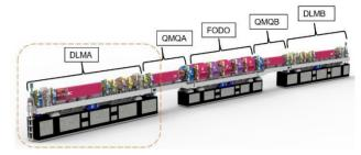
Figure 1: Typical APSU arc sector. DLMA Module (circled above) used for the first practice assembly.
