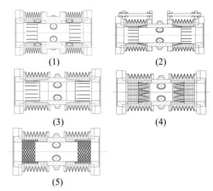
Figure 1: Shield plans of BPM bellow.
