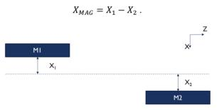
Figure 2: Top-down view of the mirror system showing absolute motion of each mirror with respect to the beam in the X direction.
