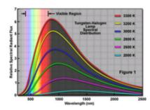
Figure 2: IR lamp flux spectrum.
