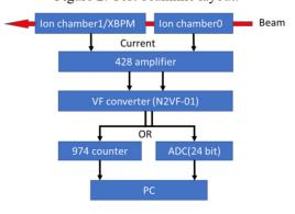
Figure 3: Data acquisition equipment.
