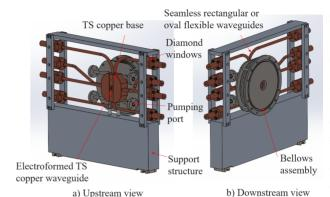
Figure 2: Transition section and its components for the compact collinear wakefield accelerator.
