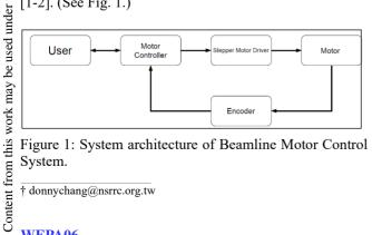
Figure 1: System architecture of Beamline Motor Control System.
