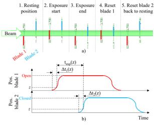
Figure 1: Exposure sequence, a) schematic of the phases of the exposure cycle b) diagram of the blades trajectories.
