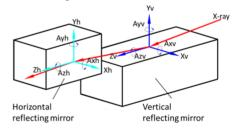
Figure 1: Schematic diagram of the K-B mirror hard X-ray nanofocusing optics.
