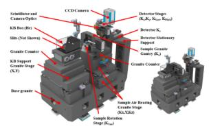
Figure 1: Rending [6] of the n-CT instrument design, labeling major components. Largest working distance (left) and probing stage (bottom right).
