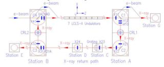
Figure 1: Schematic diagram of the CBXFEL experiment setup at the LCLS-II at SLAC.
