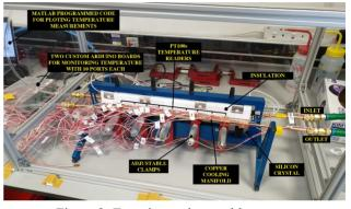
Figure 2: Experimental assembly set-up.
