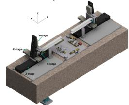
Figure 1: 3D rendering of the NSLS-II magnetic measurement system.
