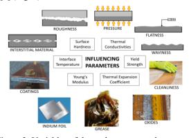
Figure 3: Variables of thermal contact conductance.
