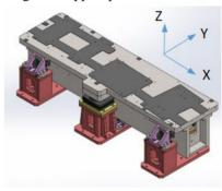
Figure 2: Girder system with three vertical support points.
