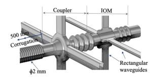
Figure 1: The corrugated waveguide and fundamental coupler followed by the IOM.
