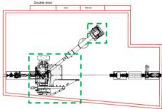
Figure 1: 8-ID-E enclosure layout with WA-XPCS instruments, diffractometer and LDDP outlined in green.
