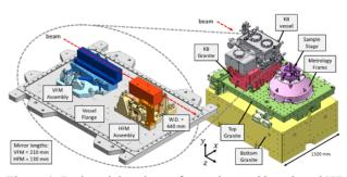
Figure 1: Reduced drawings of experimental bench and KB set with VFM and HFM assemblies in the vacuum vessel.
