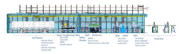
Figure 1: BioSAXS beamline schematic.
