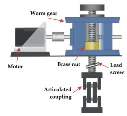
Figure 1: The drivetrain of an APS undulator device consists of a motor coupled to a 60:1 worm gear assembly. Motion is transferred to a lead screw, which is threaded through a bronze nut and connected directly to the strongback via an articulating coupling.
