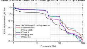
Figure 2: Integrated RMS vibration of DCM.
