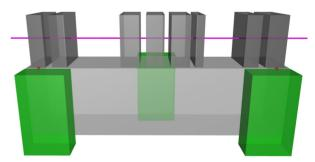
Figure 1: Model assembly including the girder design space (light gray), the magnets (dark gray), the pedestals (green), and the connection of the design space to the pedestals using beams (red). The position of the vacuum chamber is demonstrated in magenta.
