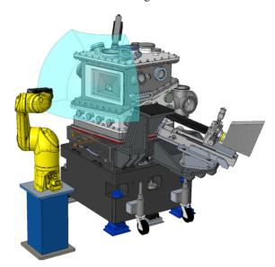
Figure 1: The new 26-ID nanoprobe enhancement as part of the advanced photon source upgrade.
