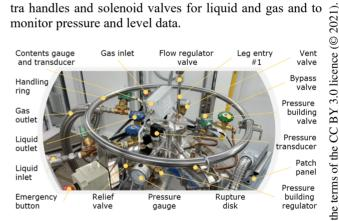
Figure 2: Top of primary LN2 cylinder and description of the connected elements.
