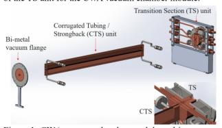
Figure 1: CWA vacuum chamber module and its components for the compact collinear wakefield accelerator.
