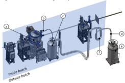
Figure 1: Third optical hutch of the CARNAUBA beamline, highlighting the liquid nitrogen supply system of the 4CM, which comprises the vacuum chamber (a), the cryostat (b), the primary (c) and secondary (e) LN2 cylinders, the transfer line (d) and the exhaust line (f).
