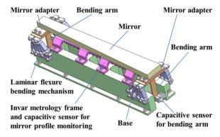
Figure 1: Photograph of the bender mirror prototype.
