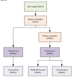
Figure 1: Cryogenics system: layered structure of hardware.
