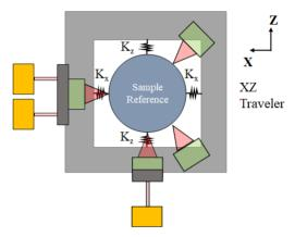
Figure 1: The coupled traveling interferometer concept. The traveling XZ travler support is coupled to the sample reference on the X and Z degrees of freedom, while decoupled in the other degrees of freedom. Focused traveling interferometers (green) and global stationary interferometers (gold) are depicted.
