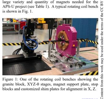
Figure 1: One of the rotating coil benches showing the granite block, XYZ-0 stages, magnet support plate, stop blocks and customized shim plates for alignment in X, Z.
