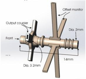
Figure 1: Model of the inner volume of a transition section, with main dimensions.
