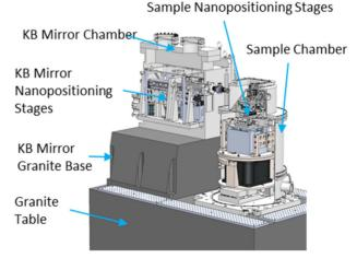
Figure 2: 3D model of the APS CSSI instrument.
