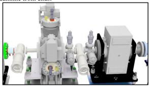
Figure 1: Rendering of the SXBPM installed in the CSX FOE as a separate section to facilitate replacement and reconfiguration of the detector assemblies.
