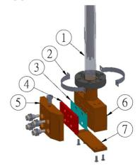
Figure 1: Internal mechanism and accessories of white beam position monitor.
