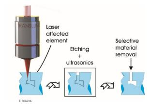
Figure 2: The two-step glass shaping process - Laser direct write, followed by selective etching.
