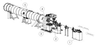
Figure 1: Main components of the endstation: (1) BCU I, (2) BCU II, (3) sample table, (4) detector gantry, and (5) flight tube.
