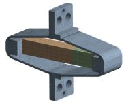
duced order model in Sim- (b) Meshed FEA model of an amplified piezoelectric actuator. Number of nodes:  $\approx 130000$ .
