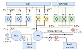
Figure 1: Simplified scheme of the ALBA's thermohydraulic cooling system.
