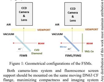
Figure 1: Geometrical configurations of the FSMs.
