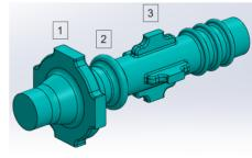
Figure 3: Geometry of the mandrel: (1) TM01 output coupler, (2) notch filter, and (3) integrated offset monitor.
