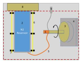
Figure 1: Schematic diagrame of the sample cryogenic cooling: 1. Crystal sample (diamond), 2. N2 reservoir, 3. crystal mount (PEEK), 4. rotation stage, 4. thermal conductor (OFHC), 5. rad. shielding (Mylar), 6. Spacer/clamps (PEEK), 7. reservoir flange (PEEK), 8. temp. sensor (RT100).
