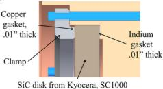
Figure 2: Design interface around SiC disk.
