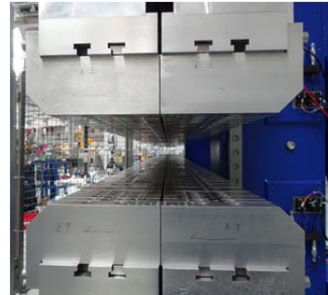
Figure 1: A common undulator configuration where there is an opening along the entire length of one side.
