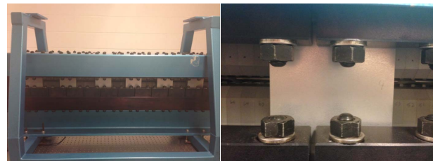
Figure 2: Left, the CSU undulator. Right, close-up of the gauge blocks fixing the magnet gap.
