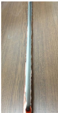
Figure 2: Test piece of the copper tube after coating (grey).
