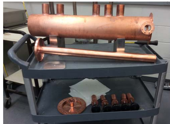
Figure 2: Cavity components before the final welding of the end plate to the outer conductor.
