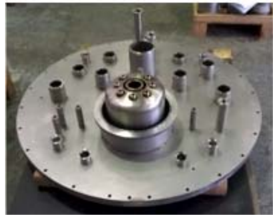
Figure 10: Prototype spoke cavity cryomodule distribution line valve box under construction.
