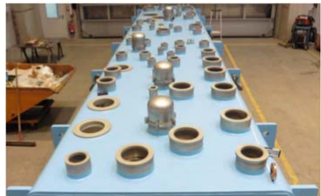
Figure 7: Machined top plate of the ACCP cold box.
