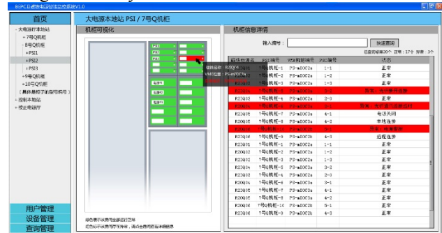
Figure 6: Visualization of the cabinets of the power supplies and the PSI chassis sitting in the cabinets.
