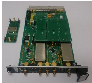
Figure 6: Transition module with filter daughter board.
