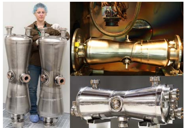
Figure 2: Left, two half-wave resonators in the cleanroom after final electron-beam welding. Top right, a half-wave resonator immediately prior to the final electron beam welding. Bottom right, a finished half-wave resonator. The HWR end-to-end length is 48 inches at room temperature.
