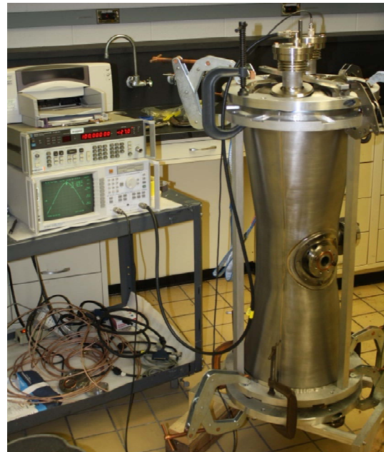
Figure 3: HWR sub-assemblies clamped together for resonant frequency measurements. The drive and pick-up probes are weakly coupled to avoid perturbing the resonant frequency.
