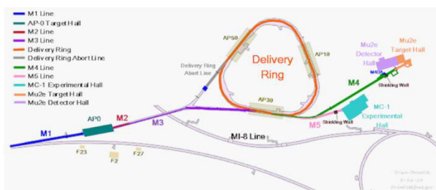
Figure 1: Layout of the Fermilab Muon Campus. Note that AP 10 is the straight section that is well aligned with the SBND detector.
