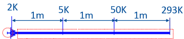
Figure 7: HOM cable cooling layout.
