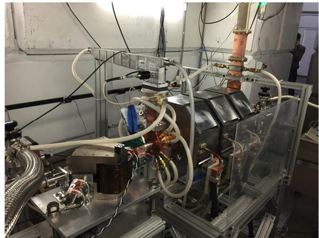
Figure 4: Assembled ARCIS linac.
