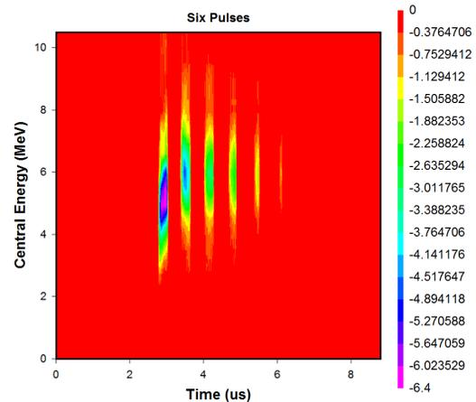
Figure 8: Time-resolved spectrum of the beam shown in Fig. 7. Color represents the beam intensity in a.u.
