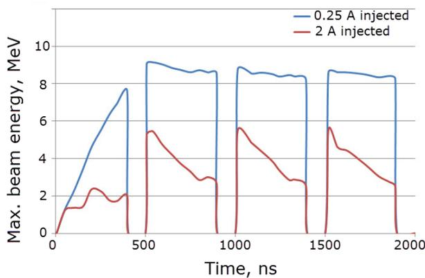
Figure 6: Temporal profile of the high (blue) and low (red) energy meso-pulses.
