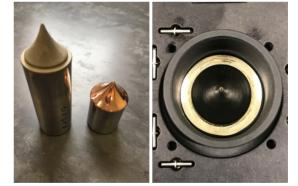
Figure 1: Butler baffles on mandrels (L) and after polishing, blackening, and mounting for optical testing (R).
