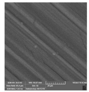
Figure 2: SEM showing texture of Acktar Spectral Black material; scale bar is 20 microns.
