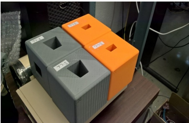
Figure 5: Block measurement fixtures / used with Helmholtz Coil.
