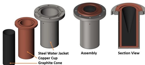
Figure 2: H + RFQ Test Stand Faraday cup components.
