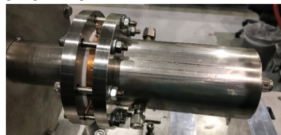
Figure 9: Faraday cup assembled at the LEBT end.
