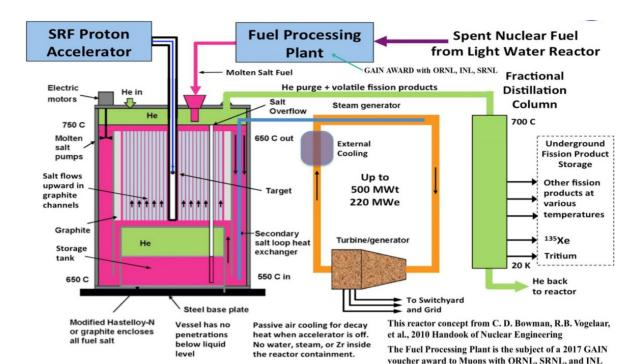
Figure 2: Conceptual diagram of the Mu\*STAR system, comprised of a 1 GeV, 2.5 MW SRF proton linac, a 500 MWt graphite moderated reactor with internal solid metal spallation neutron target, a molten-salt fuel preparation plant, and collection system for volatile radioisotopes. The reactor power can be used for process heat or electricity generation.
