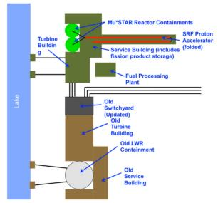
Figure 1: Mu\*STAR installed at an old LWR site.
