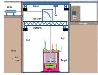
Figure 3: Underground placement of Linac and reactor.
