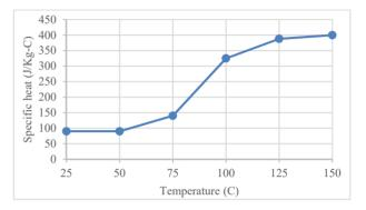
Figure 6: Specific heat, C of  $Ga_4Ni$  obtained from the test and FEA.
