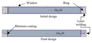
Figure 1: *Ga*<sub>4</sub>*Ni* target in Niobium capsule.
