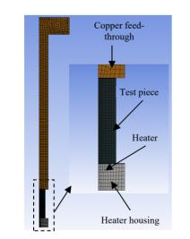
Figure 5: Axisymmetric finite element model of the test.
