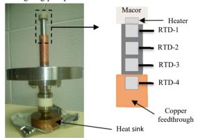
Figure 3: *Ga*<sub>4</sub>*Ni* test piece preparation for the test.
