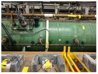
Figure 3: Detector placement for first test. The brick on the front has a 1 cm hole to act as a collimator and limit the detector's field to only one gap of the cavity. This threebrick housing proved ineffective in shielding the detectors from X-rays being produced in adjacent gaps.
