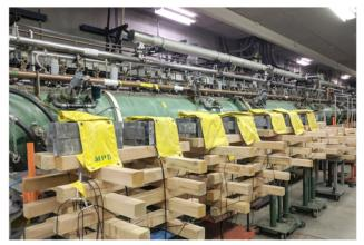
Figure 4: Lead blanket added to shield the detectors from backscattered X-rays emanating from adjacent cavities and final configuration of the detectors.
