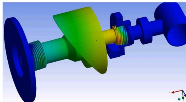
Figure 4: Mechanical model of the articulated FPC, showing the central DN100 6-inch conflat flange pair (middle of the figure). A section of beam pipe is shown in blue in the upper right side of the figure and the large insulating vacuum tank flange is shown on the left.
