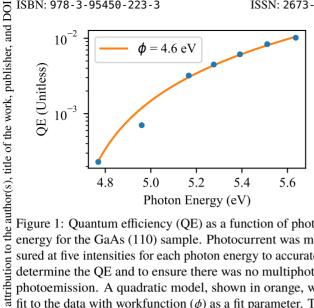
Figure 1: Quantum efficiency (QE) as a function of photon energy for the GaAs (110) sample. Photocurrent was measured at five intensities for each photon energy to accurately determine the QE and to ensure there was no multiphoton photoemission. A quadratic model, shown in orange, was fit to the data with workfunction ( $\phi$ ) as a fit parameter. The fit value of the workfunction was  $\phi = 4.6 \text{ eV}$ .
