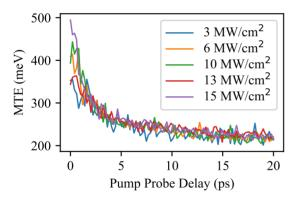
Figure 4: MTE as pump probe delay is changed at different probe intensity. Pump intensity was held at a constant  $2 \text{ MW/cm}^2$ . The MTE does change by a small amount, but only for delays where the pump and probe overlap each other.
