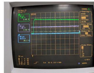
Figure 7: Scope trace showing detector prototype with modified peak detector.
