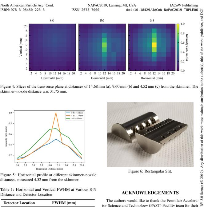
Figure 4: Slices of the transverse plane at distances of 14.68 mm (a), 9.60 mm (b) and 4.52 mm (c) from the skimmer. The skimmer-nozzle distance was 31.75 mm.
