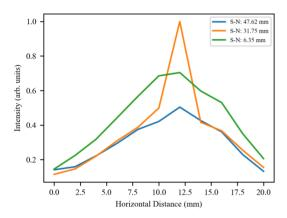
Figure 5: Horizontal profile at different skimmer-nozzle distances, measured 4.52 mm from the skimmer.
