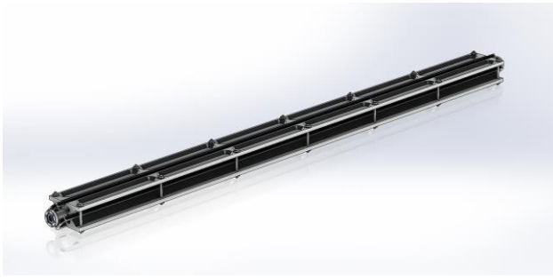
Figure 3: Current design of the AGU strongback and quadrupole configuration.
