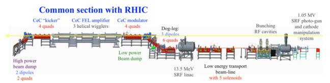
Figure 1: Layout of the CeC proof-of-principle system at IP2 of RHIC.
