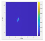
Figure 2: Image of the compressed and accelerated beam in the dogleg profile monitor. The dispersion is 1.2 meters and beam energy spread is  $3x10^{-3}$ .
