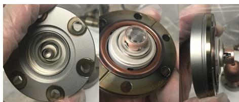
Figure 5: Left: cathode back contacts. Middle: cathode grid and emitting surface. Right: visible heater element.
