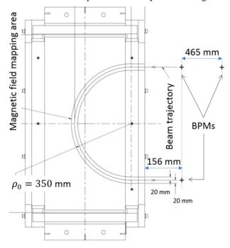
Figure 2: Schematics of 180° bend.
