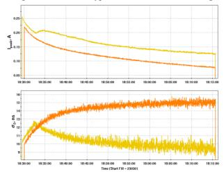
Figure 4: Typical observation of bunched electron cooling. The upper plot shows evolution of peak current of cooled (yellow trace) and test (orange trace) ion bunches. The lower plot shows evolution of the rms bunch length of the cooled and the test ion bunches during RHIC store.
