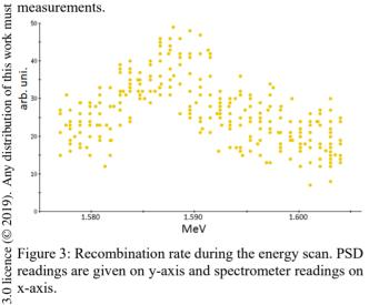
Figure 3: Recombination rate during the energy scan. PSD readings are given on y-axis and spectrometer readings on x-axis.
