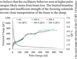
Figure 2: Extracted charge vs laser pulse energy and corresponding QE% for 0, 100 and 200 A cathode solenoid currents (225 kV, 50 kHz, 75 ps (FWHM), 1.64 mm (rms)).
