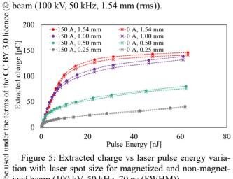
Figure 5: Extracted charge vs laser pulse energy variation with laser spot size for magnetized and non-magnetized beam (100 kV, 50 kHz, 70 ps (FWHM)).
