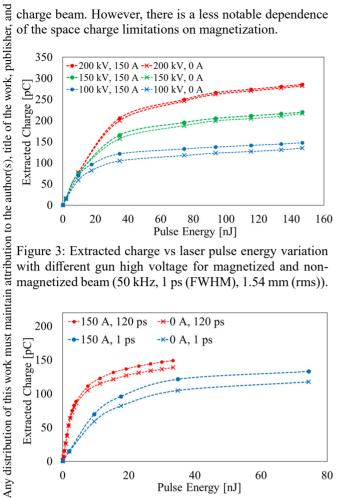
Figure 3: Extracted charge vs laser pulse energy variation with different gun high voltage for magnetized and nonmagnetized beam (50 kHz, 1 ps (FWHM), 1.54 mm (rms)).
