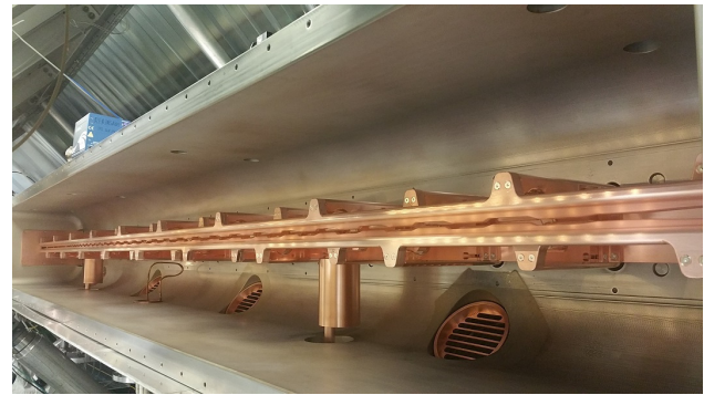
Figure 9: New ReA3 RFQ structure.
