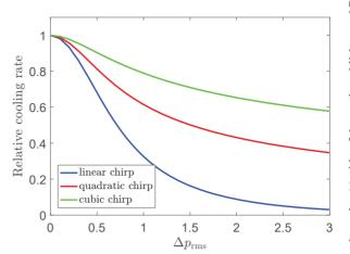
Figure 4: Relative cooling rate versus  $\Delta p_{\rm rms}$  for the three different chirp profiles (two plasma stages, case I with all chicane strengths positive).
