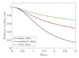
Figure 3: Relative cooling rate versus  $\Delta p_{\rm rms}$  for three different chirp profiles (no plasma stages).
