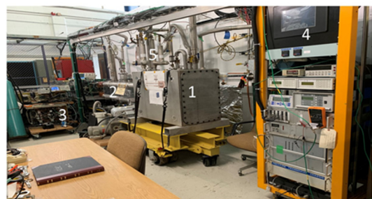
Figure 6: HTS magnet test set-up.
