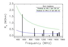
Figure 1: Thresholds of longitudinal instability for APS and APS-U.
