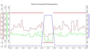
Figure 6: The frequency (red circles) and amplitude of the highest (brown) and the 2nd highest (green) spectral peaks for hor. non-dispersive BPMs. The 19-ID (NYX) undulator gap (blue) is fully opened and then fully closed.
