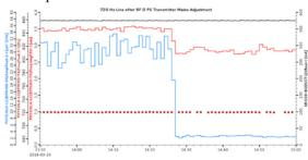
Figure 3: The amplitude of the highest spectral peak (blue), the frequency of that peak (720 Hz, brown circles), and the rms noise amplitude (red) for horizontal dispersive BPMs during cavity D RF transmitter power supply "mains compensation". 375 mA top-off current is shown in black.
