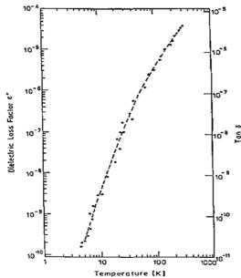
Figure 5: Dielectric loss factor and tangent delta of sapphire at 2.45 GHz vs temperature [7].
