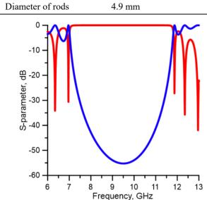
Figure 8: Reflection (red curve) and transmission (blue) characteristics of Bragg reflector vs frequency for N=8 layers.
