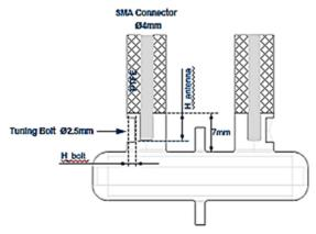
Figure 3: Drawing of X-band copper cavity.
