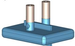
Figure 1: X-band copper resonator for Meissner qubit.
