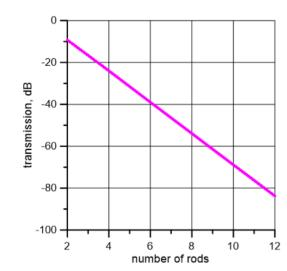
Figure 9: Transmission through Bragg reflector at central frequency of Bragg resonance vs number of rods.
