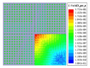
Figure 11: Structure and E-field distribution (logarithmic scale) of operating eigen mode in resonator consisted of 12 layers of rods.
