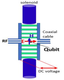
Figure 6: Sketch of sapphire resonator with SRF walls and DC electric or magnetic bias.
