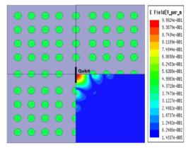
Figure 10: Structure and E-field distribution (linear scale) of operating eigen mode in resonator consisted of 4 layers of rods.
