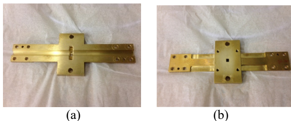
Figure 9: (a) top view and (b) bottom view of a cavity split.
