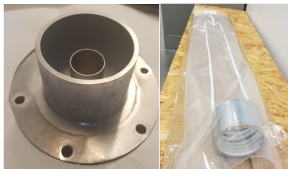
Figure 6: Secondary Sn source and the heater
