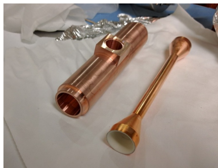
Figure 5: The fabricated dielectric structure with copper coating (right) and the copper jacket (left). High power RF flanges will be brazed onto the jacket. The opening at the jacket center is designed for pumping.
