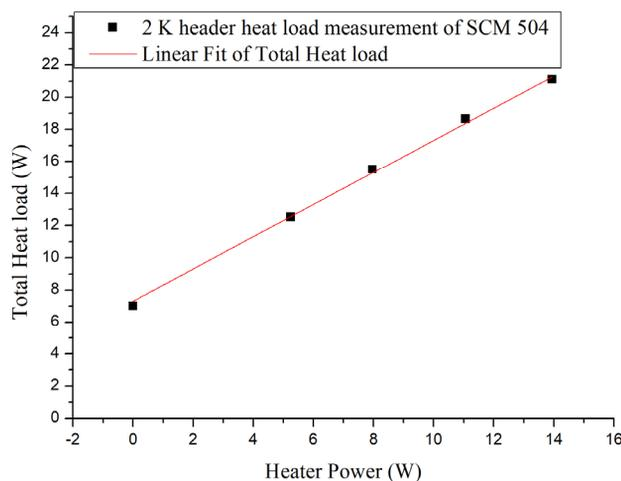
Figure 3: The cryomodule SCM 504 static heat load testing with 2 K heater calibrations.
