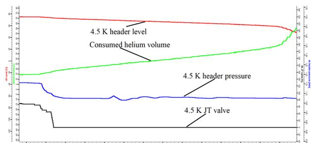
Figure 4: The 4.5 K header's heat load testing of cryomodule SCM 504.
