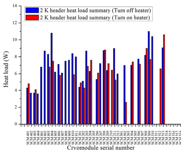
Figure 5: The 2 K header static heat load summary of FRIB cryomodule.
