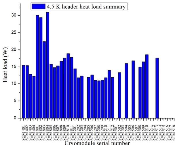
Figure 6: The 4.5 K header static heat load summary of FRIB cryomodule.
