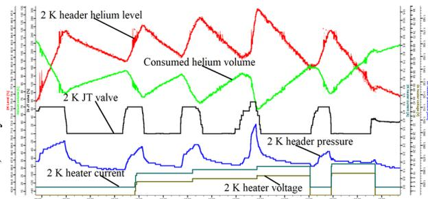
Figure 2: The 2 K header static heat load measurement of SCM 504.
