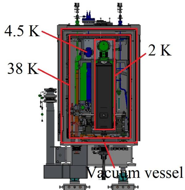
Figure 1: The section view of 0.085 cryomodule of FRIB.
