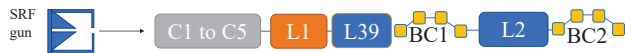
Figure 5: Diagram of the photoinjector and linac used in the simulations to produce the tailored bunch. The injector consists of a SRF gun and a 650-MHz linac (C1 to C5). L1 and L2 are 650 MHz linacs, L39 is a 3.9-GHz linac, and BC1 and BC2 are magnetic bunch compressors.
