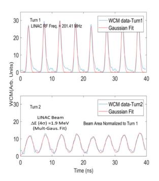
Figure 2: (a) Bunch profiles for  $1^{st}$  turn in the Booster and (b) multi-Gaussian fit for WCM data for the same beam on second turn. These arbitrarily chosen eight bunches with no overlapping bunches. Measured  $\Delta E$  are also shown.
