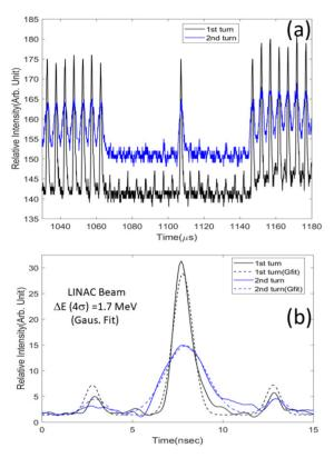
Figure 1: (a) Bunch profiles for  $1^{st}$  and  $2^{nd}$  turn in the Booster and (b) Gaussian fit to the untouched single bunch in the notch for  $1^{st}$  and  $2^{nd}$  turn. Measured  $\Delta E$  are also shown.
