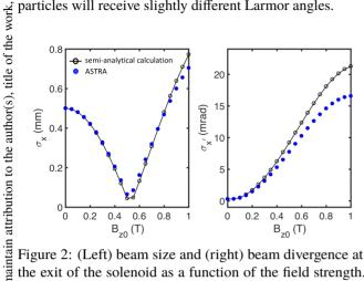
Figure 2: (Left) beam size and (right) beam divergence at the exit of the solenoid as a function of the field strength. In the numerical setup, for the solenoid  $\kappa = 0.01$  m and must  $L_{\rm sol} = 0.1$  m. The initial beam size is assumed 0.5 mm, with work the normalized emittance 1  $\mu$ m.
