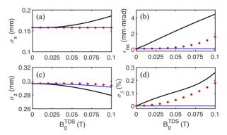
Figure 3: Dependence on the magnetic deflecting field for (a) beam size and; (b) beam emittance; (c) bunch length; (d) the relative energy spread, at the exit of the TDS. The black lines are obtained from our semi-analytical model, the blue lines from the analytical formulas by van Rens et al. [5], and the red dots from particle tracking simulation ELEGANT.
