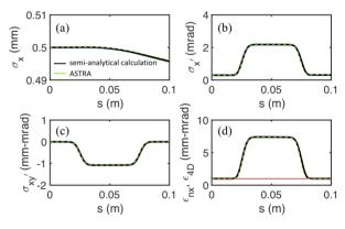
Figure 1: (a) Transverse rms beam size as a function of *s*; (b) transverse rms beam divergence as a function of *s*; (c) transverse x - y' correlation as a function of *s*; (d) transverse emittances as a function of *s*. The red line in (d) refers to the transverse 4-D emittance, which is conserved along *s*.
