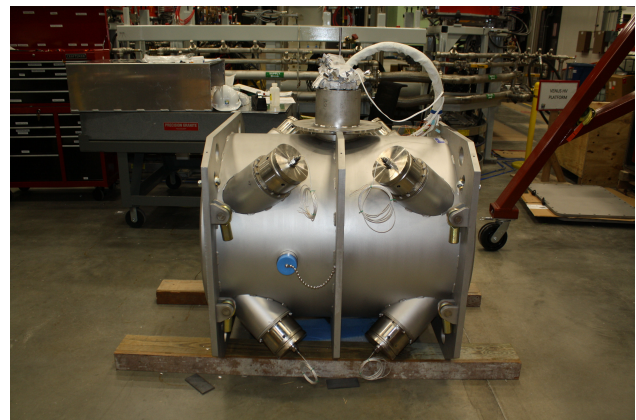
Figure 4: View of the FRIB SCECR lower cryostat assembly.
