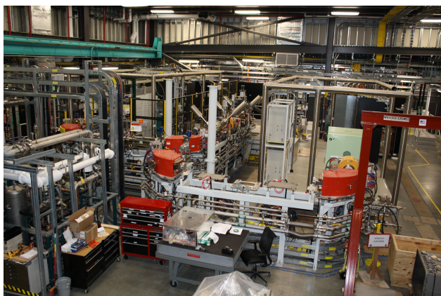
Figure 5: Layout of FRIB ECR ion sources on HV platforms. The 28 GHz source is shown at the forefront while the 14 GHz ECR ion source used for commissioning is shown at the back.
