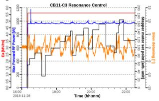
Figure 5: Resonance control of a  $\beta = 0.085$  QWR at 4.5 K. The slow detuning (orange) is the phase difference between the input and pickup RF signals, filtered by a 3 Hz low-pass filter. The peak forward RF power (blue) is measured every second with a 100 kHz bandwidth. Red: accelerating gradient. Black: stepping motor position set point.
