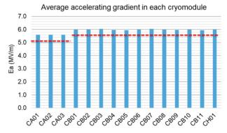
Figure 1: Accelerating gradients achieved in LS1. Solid blue bars: average accelerating gradient in each cryomodule. Dashed red lines: design gradients.
