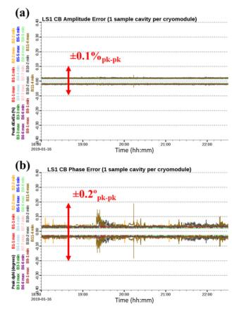
Figure 3: Measured amplitude and phase errors without beam: (a) fractional amplitude, (b) phase. The plots show the minimum or maximum value measured for every one second bin with the 100 kHz bandwidth. The horizontal time span is 5 hours. Eleven cavities in CB cryomodules are shown, i.e. one cavity per cryomodule. The other LS1 cavities show similar performance.
