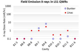
Figure 2: Field emission X-rays at design  $E_a$  for cavities with X-ray dose rates >0.1 mR/hr. The red dots (linac) were measured after opening the beam line gate valves at each end of each cryomodule.
